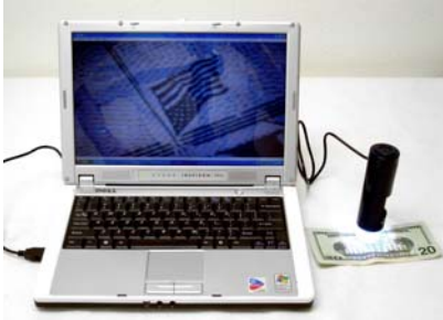
Handheld Digital Microscope with a Laptop
