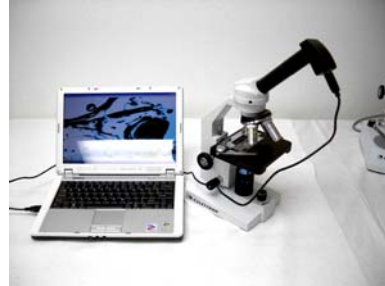
Microscope VGA Imager attached to a microscope and laptop
